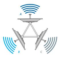
• Two APs Set the same frequency on both APs located back to back (this is the AA channel design).
