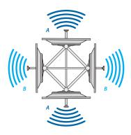
Three APs Set a different frequency on each AP (this is the ABC channel design). For example, a client is located equidistant from two APs (one set to frequency A and one set to frequency B). The client will only receive signals from the AP that shares its frequency. A different client is located equidistant from a different pair of APs (one set to frequency B and one set to frequency C). This client will only receive signals from the AP that shares its frequency.
