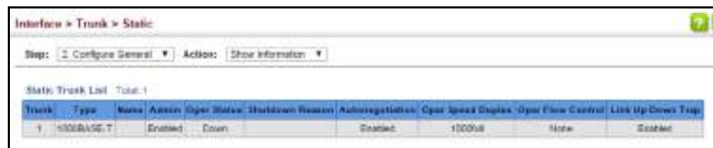
Figure 49: Showing Information for Static Trunks
