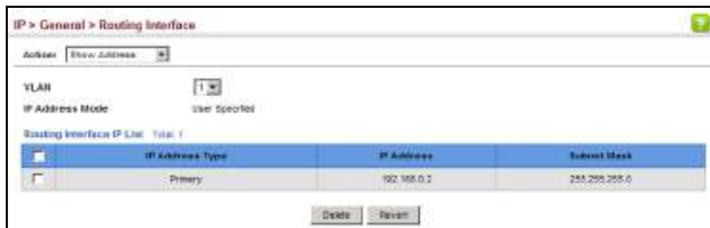
Figure 318: Showing the Configured IPv4 Address for an Interface
