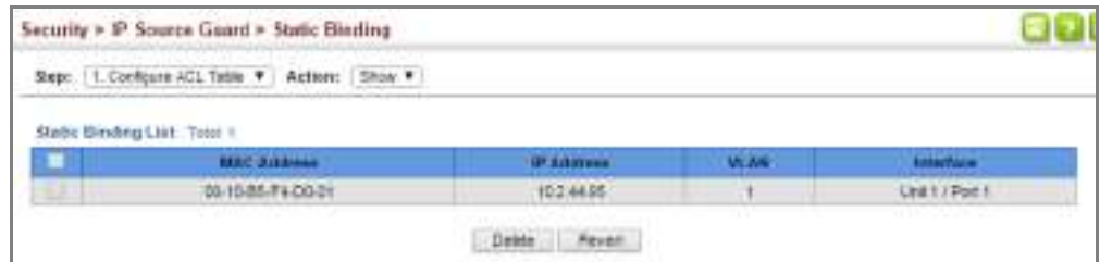
Figure 194: Displaying Static Bindings for IPv4 Source Guard
