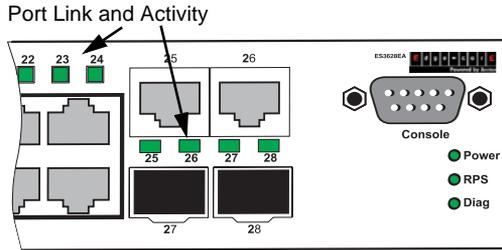
**Figure 1-2 Port LEDs**
