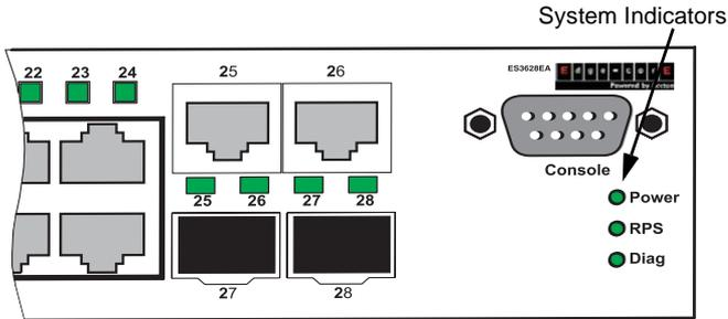
**Figure 1-3 System LEDs**
