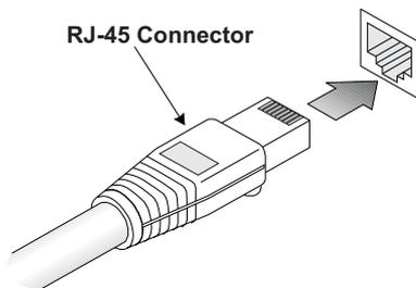
**Figure 3-1 RJ-45 Connections**
