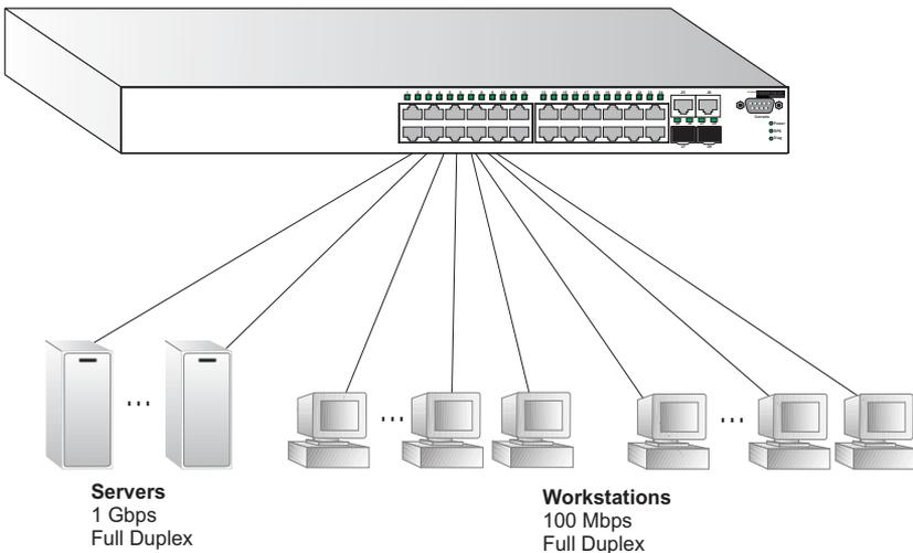
**Figure 2-1 Collapsed Backbone**
