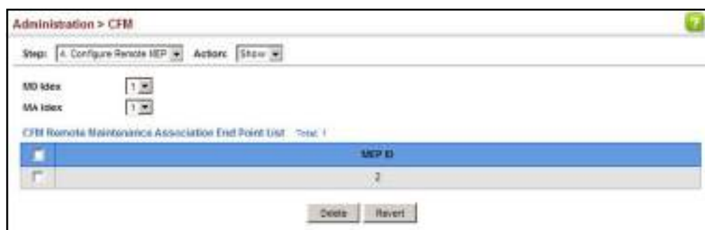
Figure 347: Showing Remote Maintenance End Points
