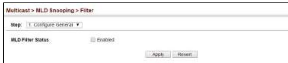
Figure 411: Enabling MLD Filtering and Throttling
