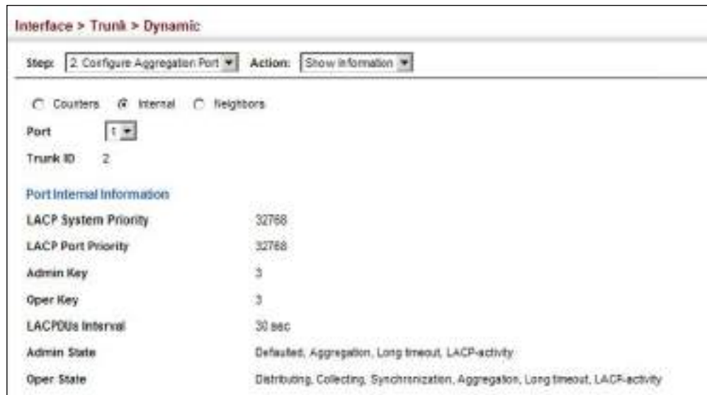
Figure 56: Displaying LACP Port Internal Information
