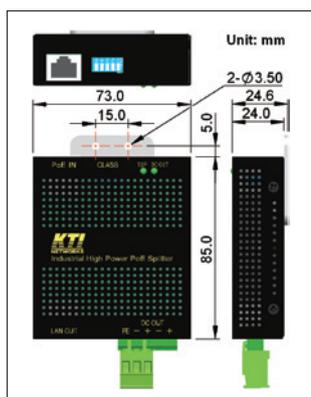
KTI Network's KPW-T2P25 is a high power PoE splitter which integrates Power over Ethernet (PoE) technology to PoE incapable network device by just using a single Cat.5 cable for both power and data transaction. The equipments such as Wireless Router, AP, Network Camera, Print server, and Media converter which connect to the PoE splitter, all devices become PoE enabled to eliminate the need of power outlets as well as cable installation and expense.
