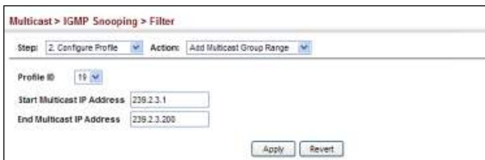
Figure 348: Adding Multicast Groups to an IGMP Filtering Profile
