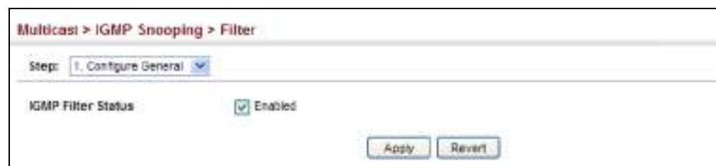
Figure 345: Enabling IGMP Filtering and Throttling
