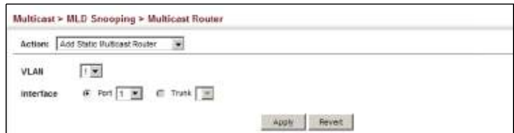
Figure 353: Configuring a Static Interface for an IPv6 Multicast Router
