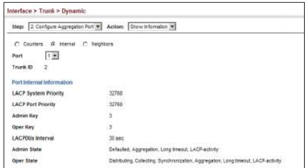
Figure 56: Displaying LACP Port Internal Information
