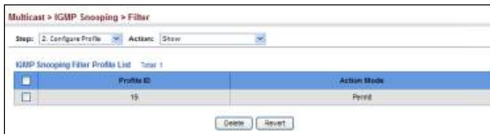
Figure 347: Showing the IGMP Filtering Profiles Created
