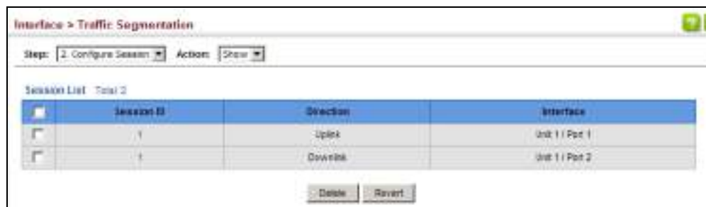
Figure 73: Showing Traffic Segmentation Members
