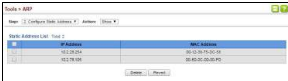
Figure 392: Displaying Static ARP Entries
