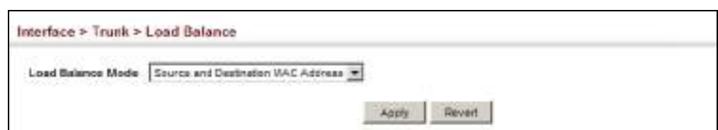
Figure 58: Configuring Load Balancing
