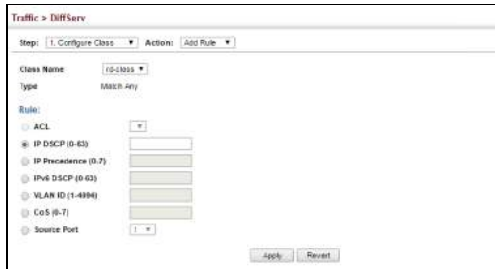
Figure 155: Adding Rules to a Class Map
