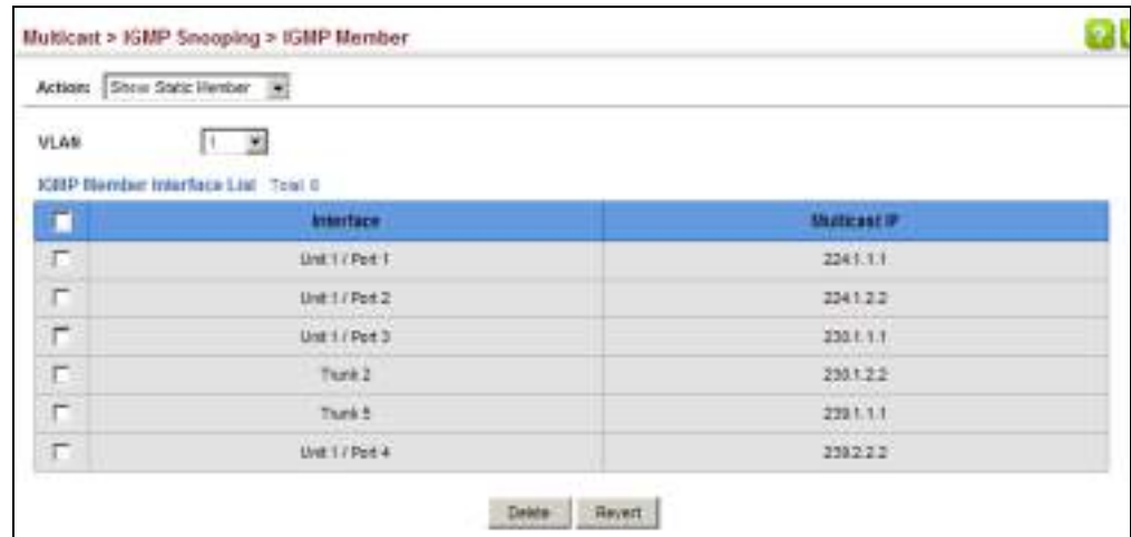
Figure 336: Showing Static Interfaces Assigned to a Multicast Service
