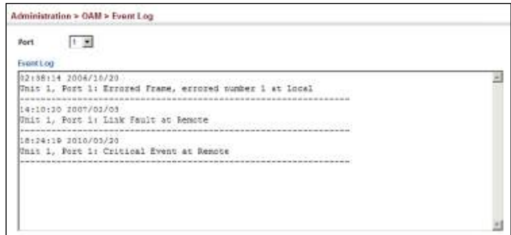
Figure 321: Displaying the OAM Event Log
