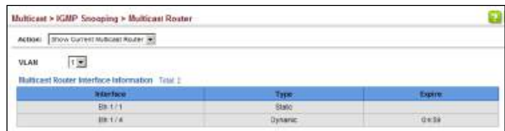
Figure 334: Showing Current Interfaces Attached a Multicast Router
