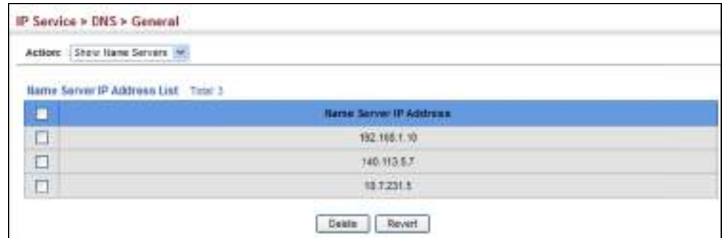
Figure 419: Showing the List of Name Servers for DNS
