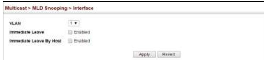
Figure 352: Configuring Immediate Leave for MLD Snooping
