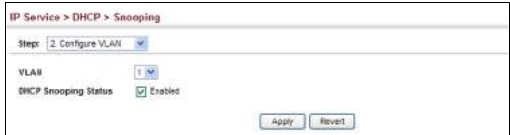
Figure 221: Configuring DHCP Snooping on a VLAN
