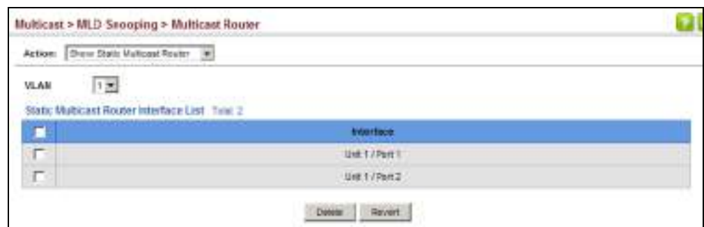
Figure 354: Showing Static Interfaces Attached an IPv6 Multicast Router
