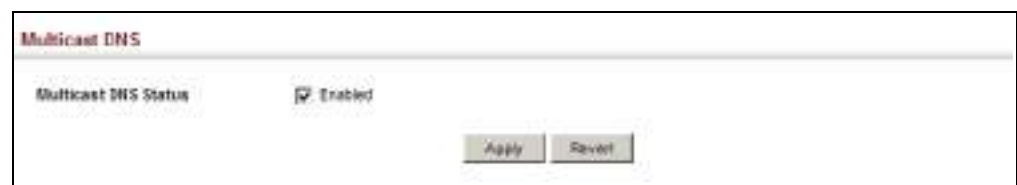
Figure 423: Configuring Multicast DNS
