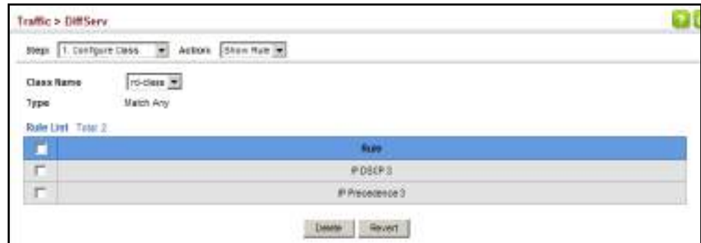
Figure 156: Showing the Rules for a Class Map
