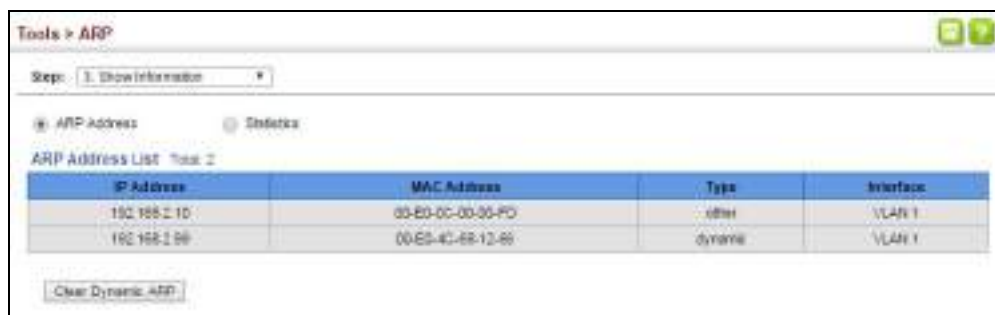
Figure 393: Displaying ARP Entries
