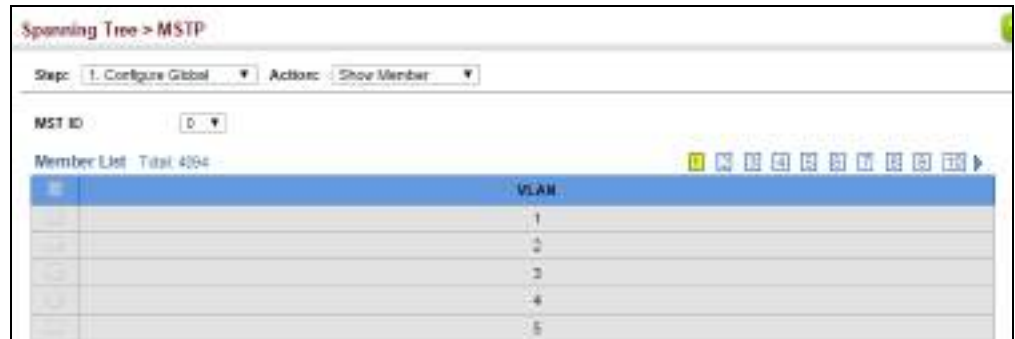
Figure 131: Displaying Members of an MST Instance
