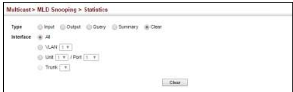
Figure 366: Clearing MLD Snooping Statistics
