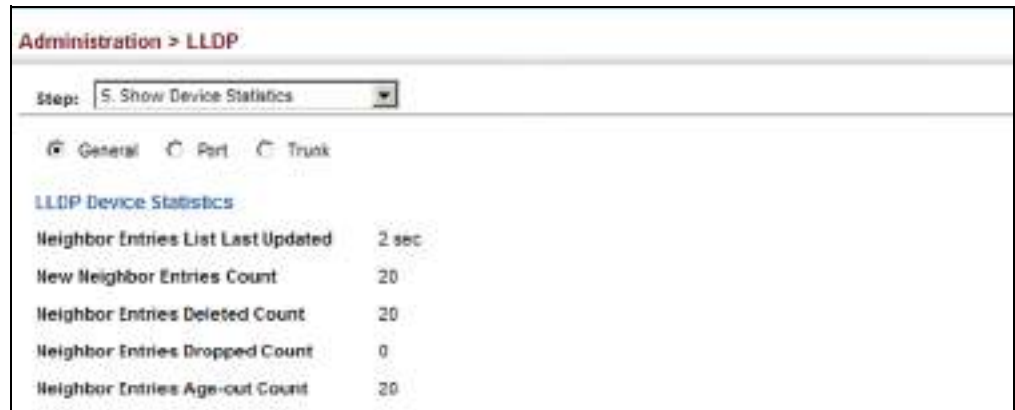
Figure 264: Displaying LLDP Device Statistics (Port)
