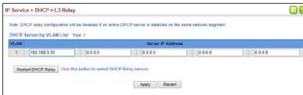
Figure 426: Configuring L3 DHCP Relay Service
