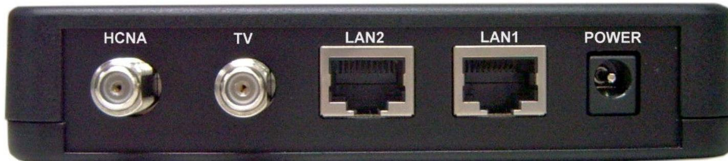
**Figure 2.2: Rear side of the Modem**
