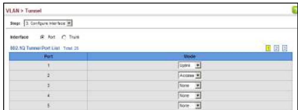
Figure 81: Adding an Interface to a QinQ Tunnel
