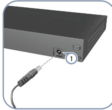
**Note:** The ECS2100-10PE includes an AC-DC power adapter. Connect the AC-DC power adapter to the switch and to an AC power source. The AC-DC adapter provides 54 VDC, 1.67 A of power to the switch.
