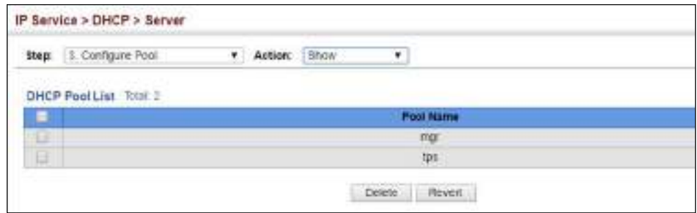
Figure 492: Showing Configured DHCP Server Address Pools
