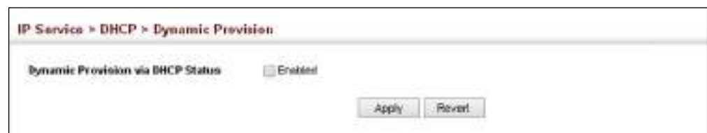
Figure 485: Enabling Dynamic Provisioning via DHCP
