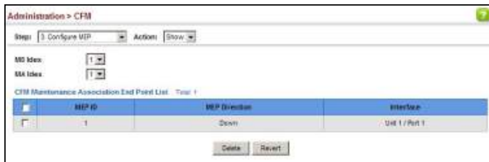
Figure 345: Showing Maintenance End Points
