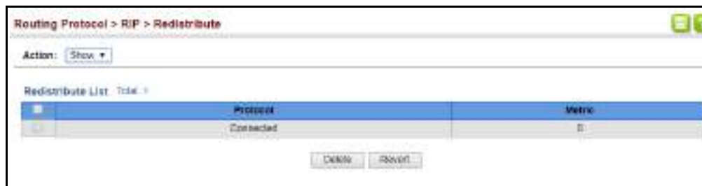
Figure 350: Showing External Routes Redistributed into RIP
