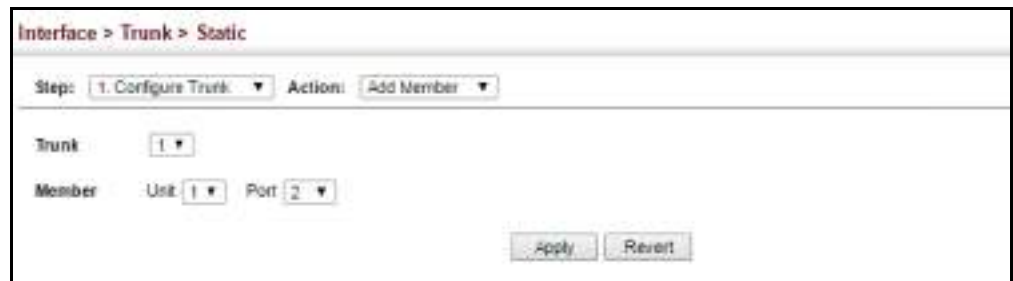
Figure 46: Adding Static Trunks Members
