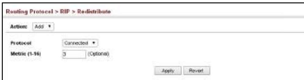
Figure 349: Redistributing External Routes into RIP
