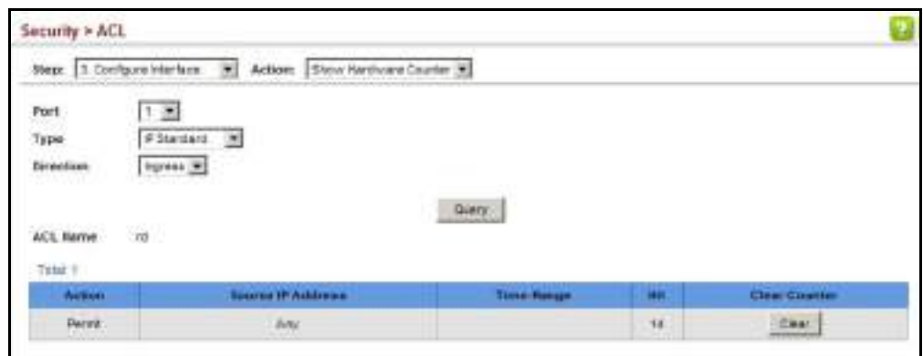
Figure 187: Showing ACL Statistics
