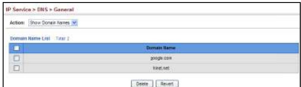
Figure 360: Showing the List of Domain Names for DNS
