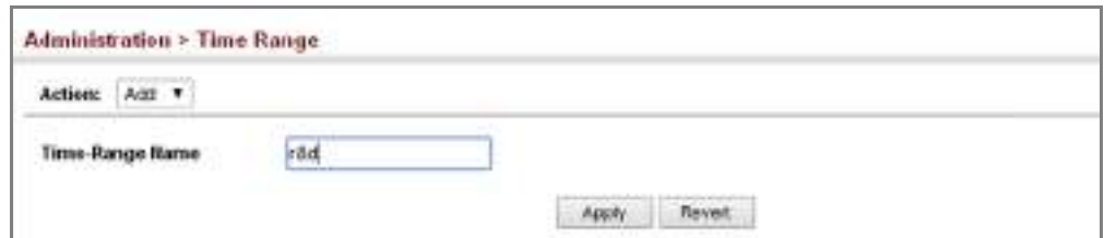
Figure 264: Setting the Name of a Time Range
