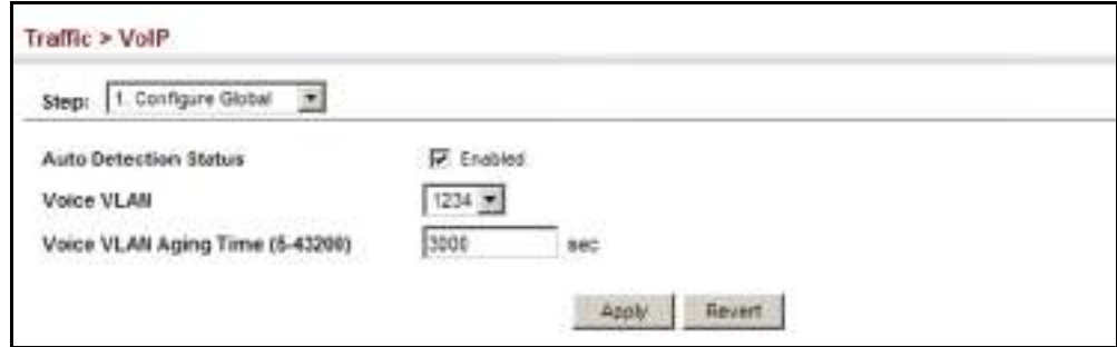
Figure 139: Configuring a Voice VLAN
