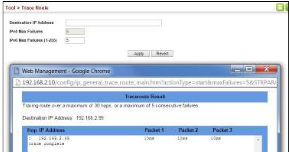
Figure 317: Tracing the Route to a Network Device
