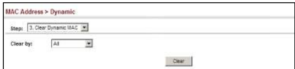
Figure 94: Clearing Entries in the Dynamic MAC Address Table
