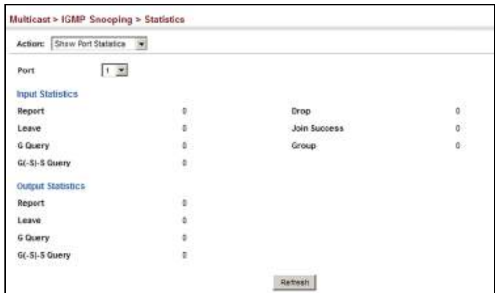
Figure 287: Displaying IGMP Snooping Statistics – Port
