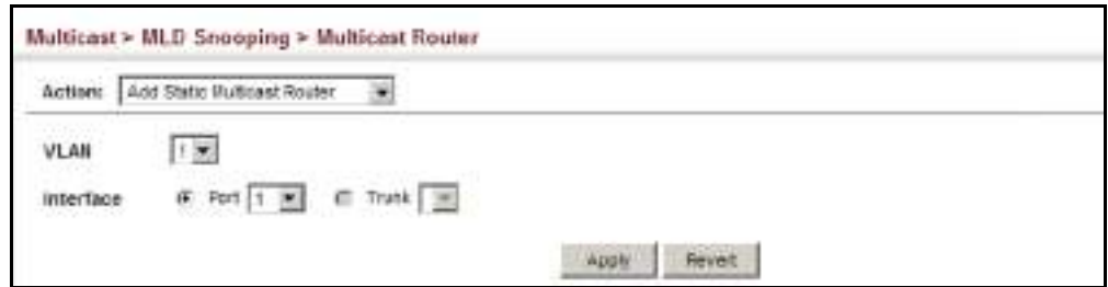
Figure 296: Configuring a Static Interface for an IPv6 Multicast Router
