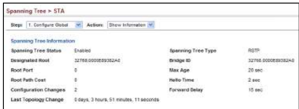
Figure 108: Displaying Global Settings for STA
