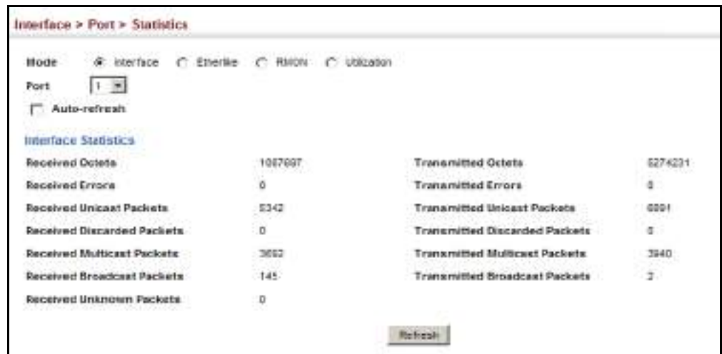
Figure 34: Showing Port Statistics (Table)
