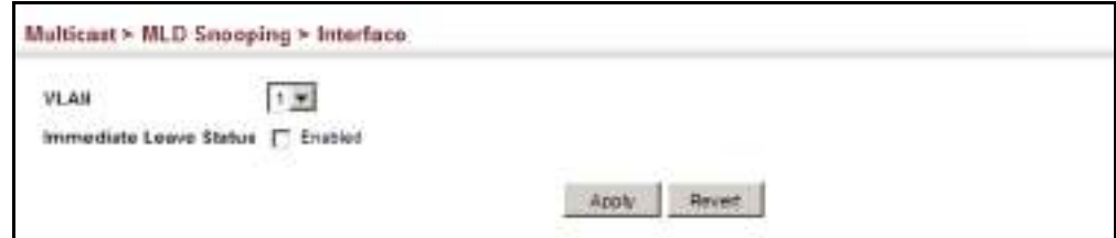
Figure 295: Configuring Immediate Leave for MLD Snooping
