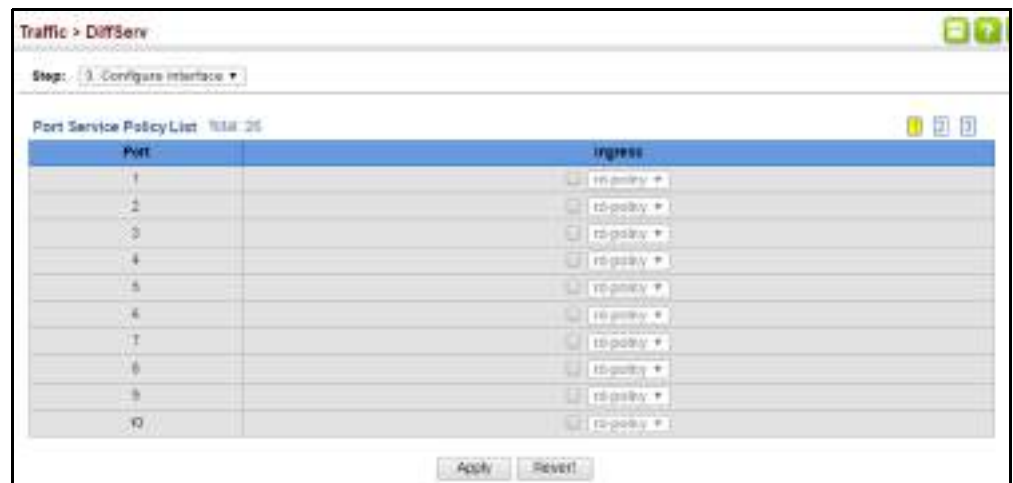
Figure 138: Attaching a Policy Map to a Port
