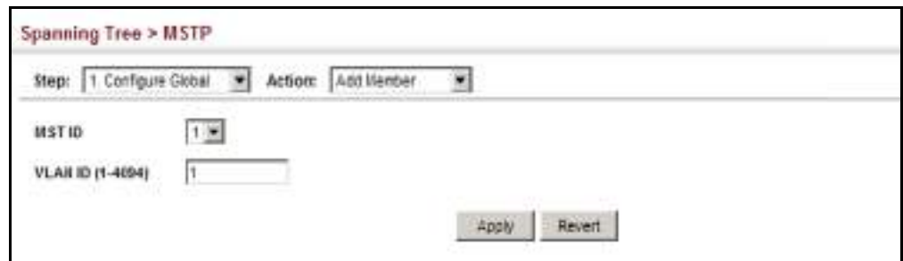
Figure 117: Adding a VLAN to an MST Instance
