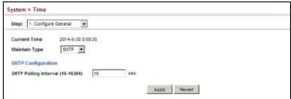
Figure 12: Setting the Polling Interval for SNTP
