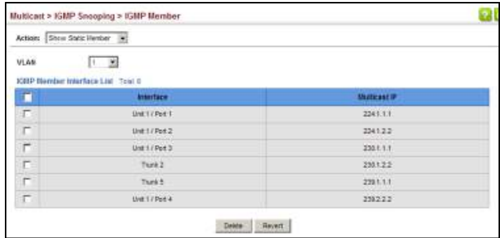
Figure 280: Showing Static Interfaces Assigned to a Multicast Service
