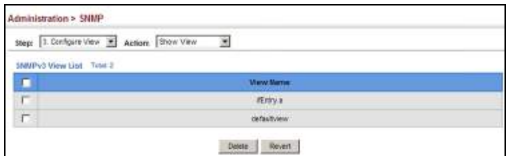
Figure 230: Showing SNMP Views
