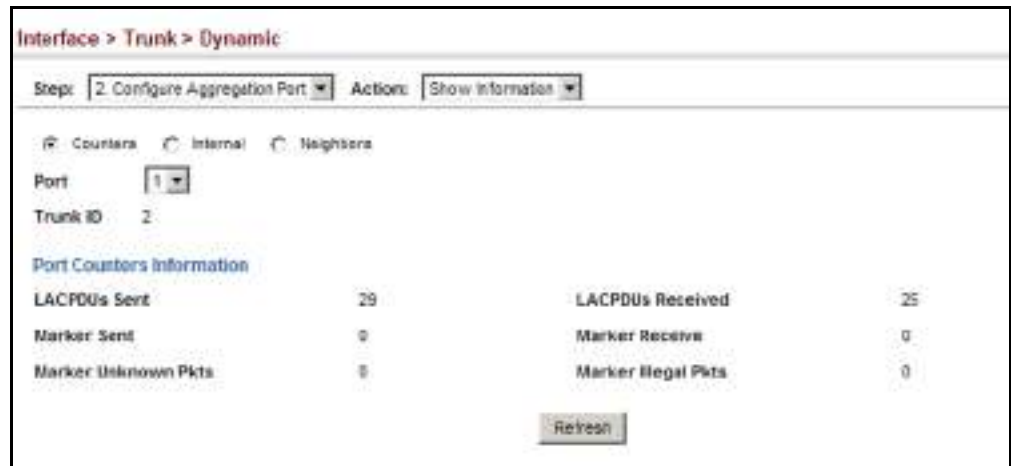
Figure 56: Displaying LACP Port Counters
