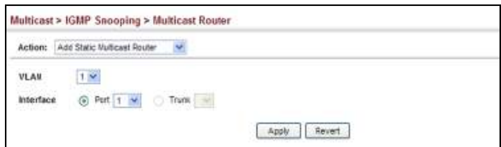
Figure 276: Configuring a Static Interface for a Multicast Router
