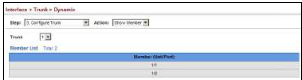
Figure 53: Showing Members of a Dynamic Trunk
