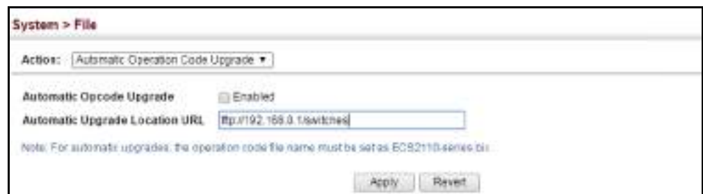
Figure 10: Configuring Automatic Code Upgrade
