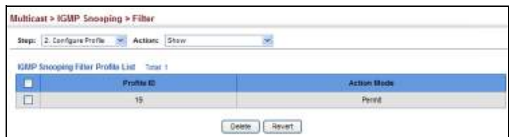
Figure 290: Showing the IGMP Filtering Profiles Created
