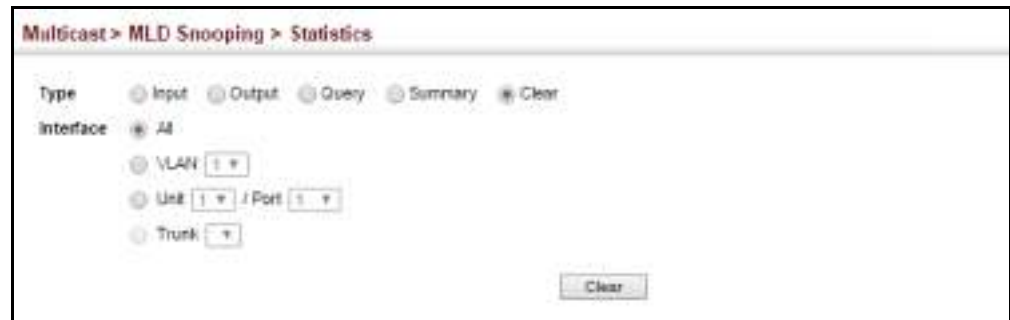
Figure 308: Clearing MLD Snooping Statistics
