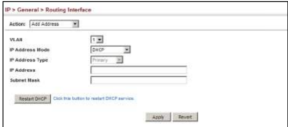
Figure 325: Configuring a Dynamic IPv4 Address
