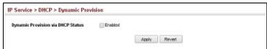
Figure 370: Enabling Dynamic Provisioning via DHCP
