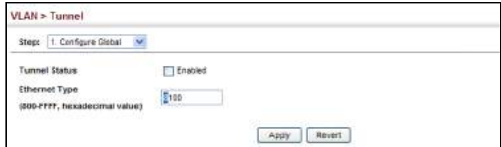
Figure 83: Enabling QinQ Tunneling
