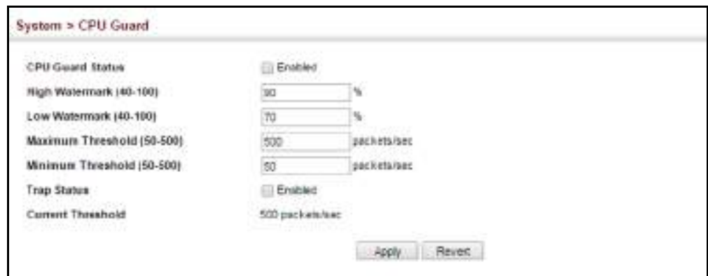
Figure 24: Configuring CPU Guard
