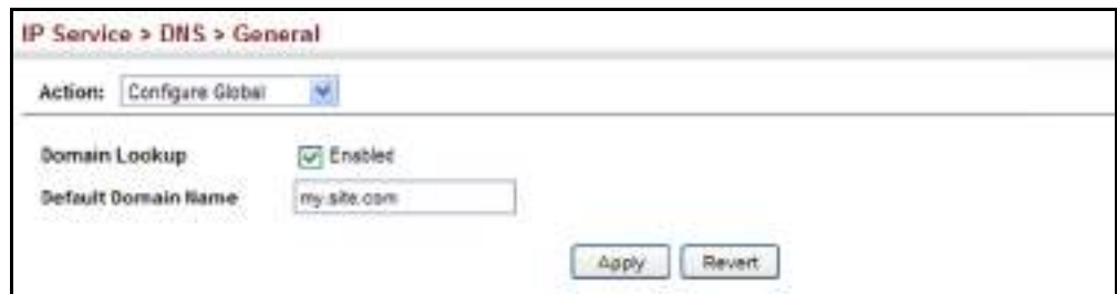
Figure 358: Configuring General Settings for DNS
