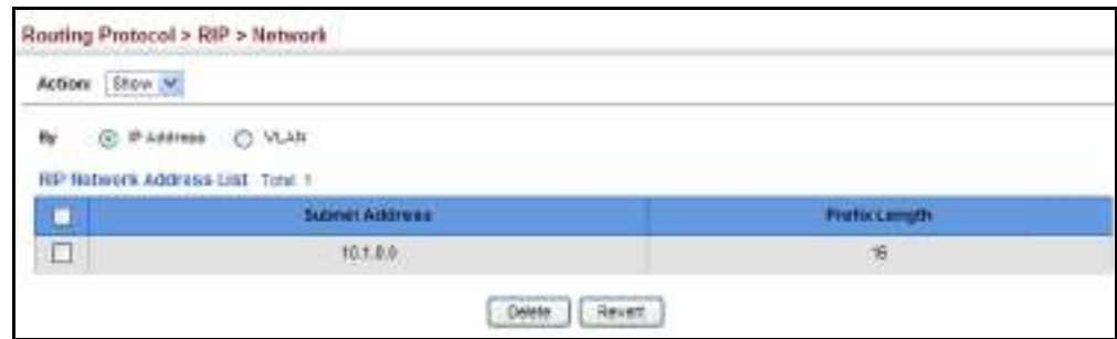
Figure 344: Showing Network Interfaces Using RIP
