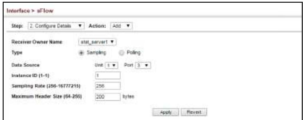
Figure 70: Configuring an sFlow Instance
