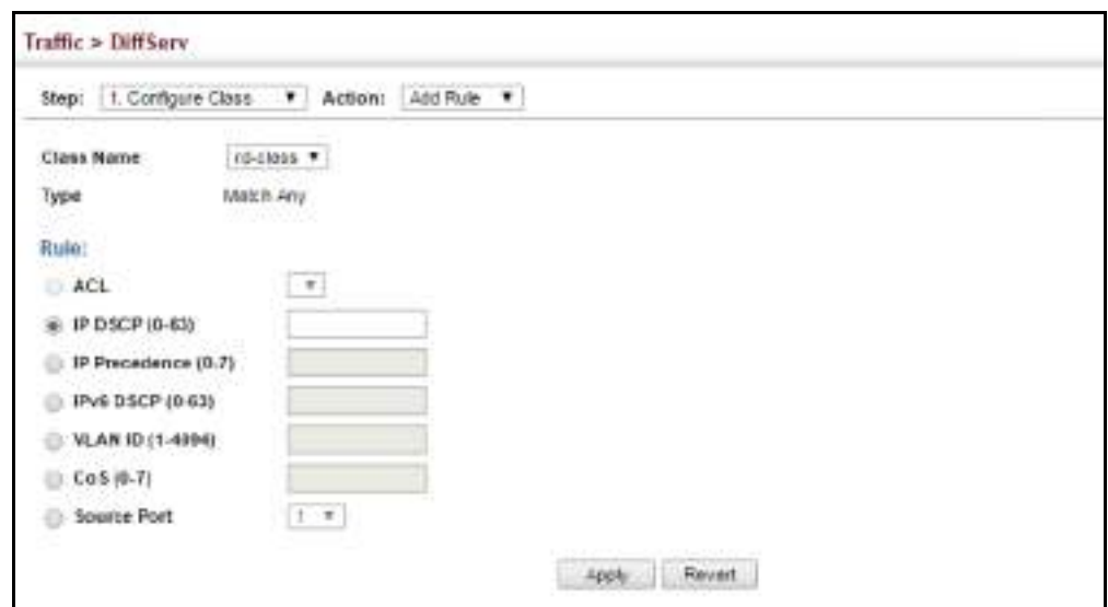
Figure 132: Adding Rules to a Class Map
