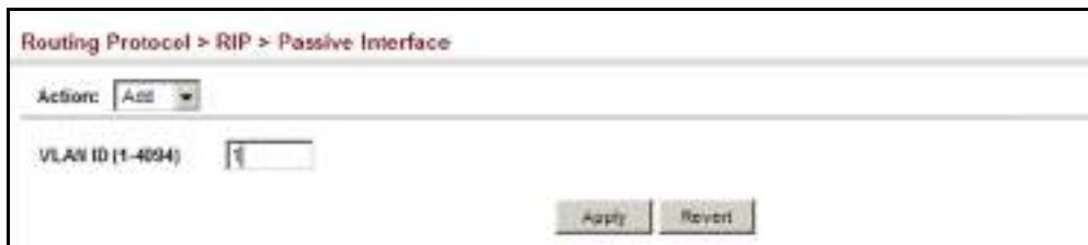
Figure 345: Specifying a Passive RIP Interface
