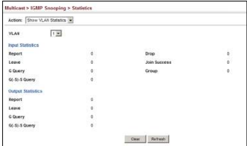
Figure 286: Displaying IGMP Snooping Statistics – VLAN
