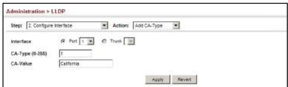
Figure 215: Configuring the Civic Address for an LLDP Interface
