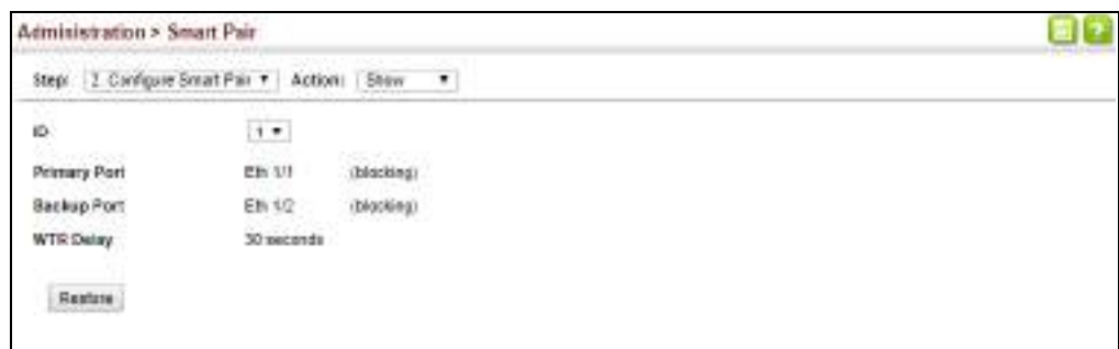
Figure 273: Displaying Port Members of a Smart Pair
