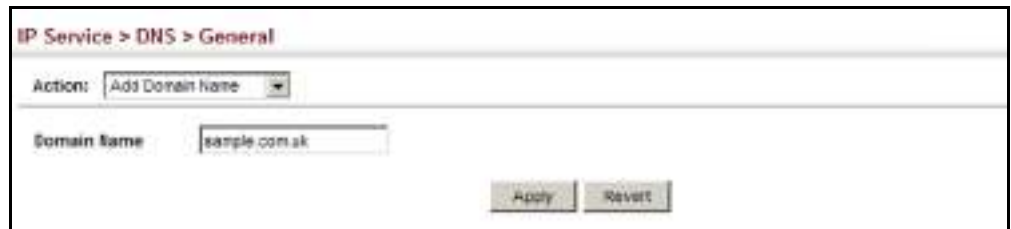
Figure 359: Configuring a List of Domain Names for DNS
