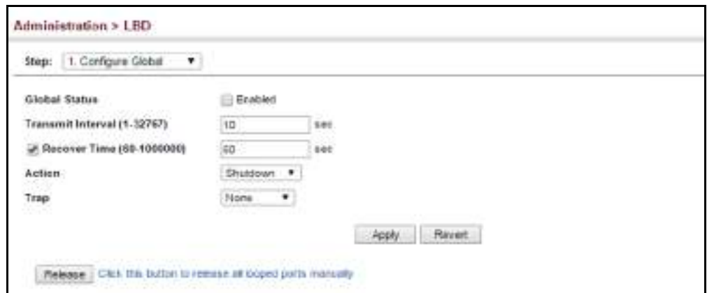
Figure 268: Configuring Global Settings for LBD
