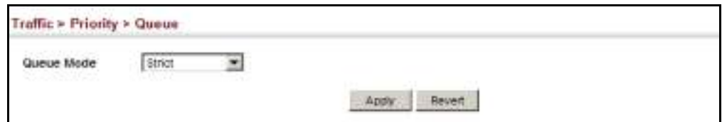
Figure 125: Setting the Queue Mode (WRR)
