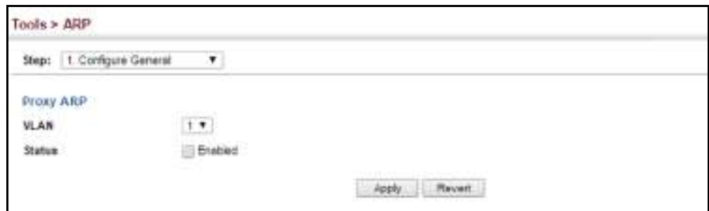
Figure 319: Configuring General Settings for ARP
