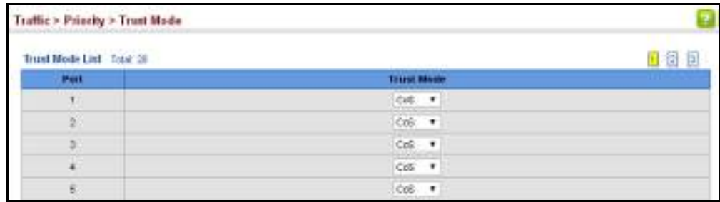
Figure 127: Setting the Trust Mode
