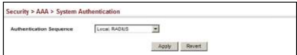
Figure 143: Configuring the Authentication Sequence
