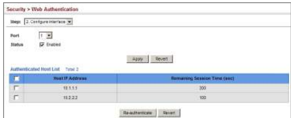
Figure 164: Configuring Interface Settings for Web Authentication
