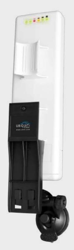
Mount with window mount adapter attached to NanoStation.
