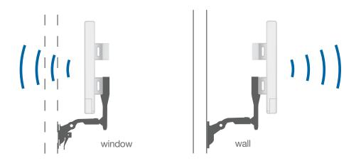
The kit comes with interchangeable mounting adapters (suction mount for window, wall screws for wall) so the NanoStation can be easily fitted on a window or wall.
