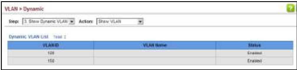
Figure 76: Showing Dynamic VLANs Registered on the Switch
