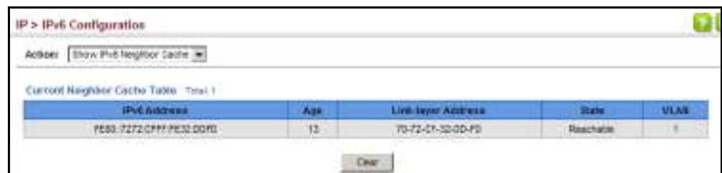
Figure 335: Showing IPv6 Neighbors
