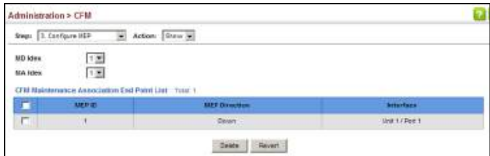
Figure 302: Showing Maintenance End Points
