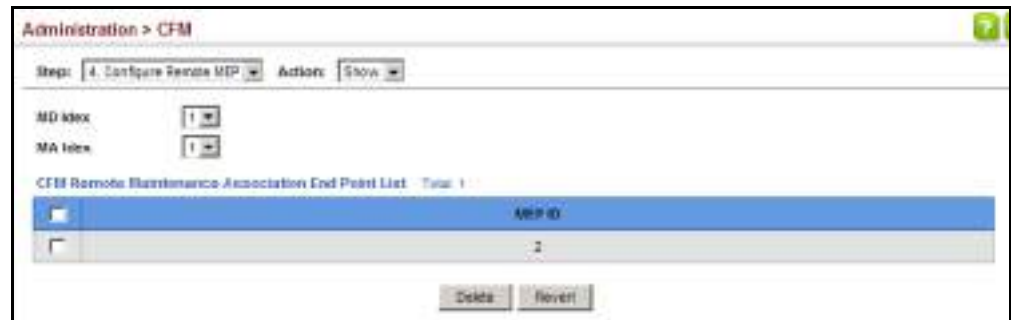
Figure 304: Showing Remote Maintenance End Points
