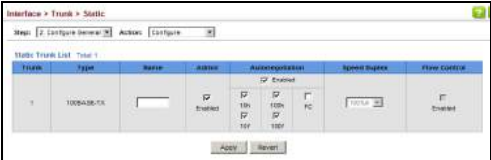
Figure 47: Configuring Connection Parameters for a Static Trunk
