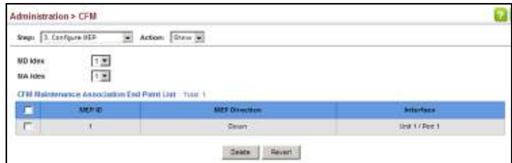
Figure 325: Showing Maintenance End Points
