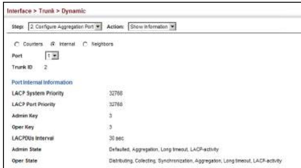
Figure 57: Displaying LACP Port Internal Information
