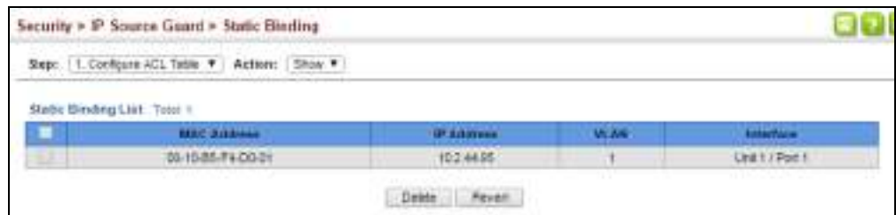
Figure 231: Displaying Static Bindings for IPv4 Source Guard
