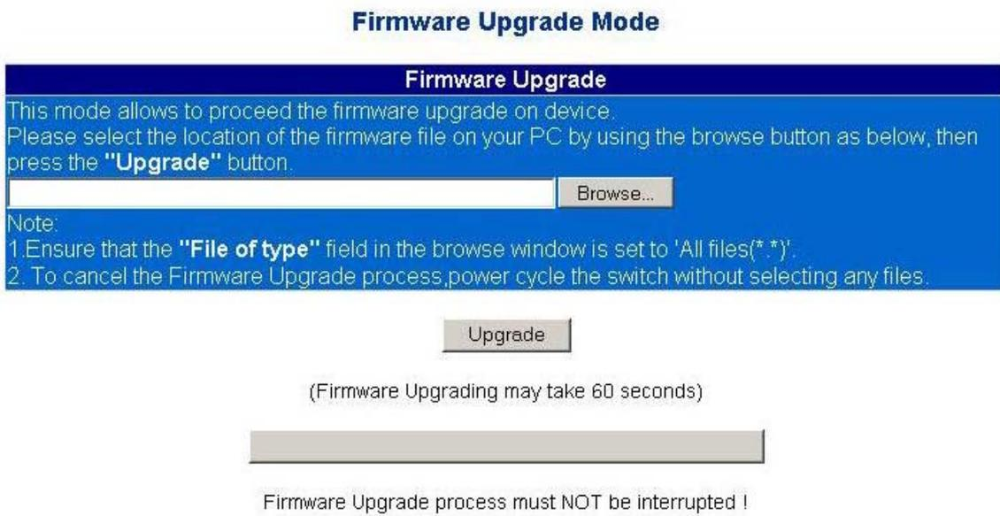
Figure 4-10 Firmware Upgrade screen
