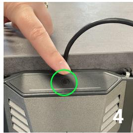
4. Start the Sidekick by **pressing the on/off switch for at least 2 seconds**. The LED bar lights up in colour from right to left and the Sidekick starts. When the LED bar lights up blue (not yet connected by cable) or green (already connected by cable), the Sidekick is ready for operation.
